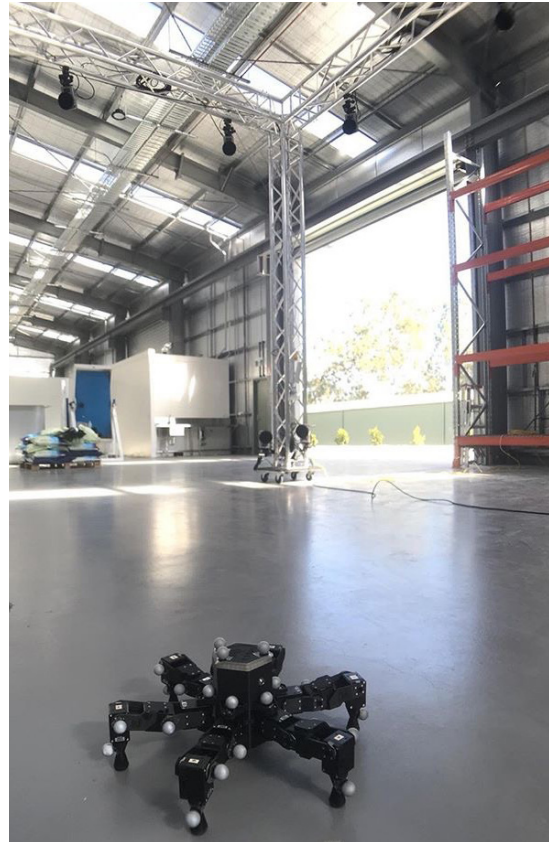
An autonomous hexapod at CSIRO inspects & maps ceiling cavity and underfloor as Qualisys cameras track it.
